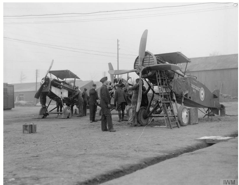
Air mechanics working on reconnaissance aircraft at the aircraft repair depot near Rang du Fliers, Northern France, July 1918. The canvas covering stretched over the framework of the aircraft can be clearly seen. © IWM (Q11963)
