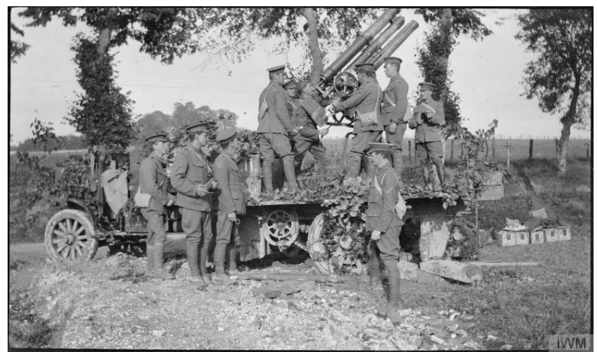
Lorry mounted 13-pounder anti-aircraft gun of No.11 Anti-Aircraft Section, Royal Garrison Artillery, ready for action, 1915. © IWM (HU 108149)
